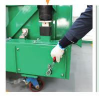
Mechanical Deck angle adjustable while working system to work reliably for different drilling fluids
